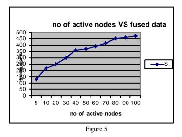
In The Figure 5 We See That The Fusing Data Of Clusters Changes With The Total Number Of Active Nodes In The Entire Network. As The Total Number of Actives Nodes Increase, The Number Of Fusing Data Also Increases
